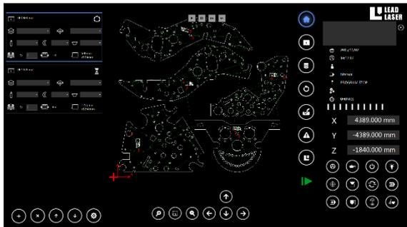
All tasks for the machine can be managed, organized and visualized in the task manager. PRC Lead Laser Suite© will provide the operator with all necessary information about the correct set-up of the machine. When used with automatic loading and unloading equipment, the task manager will make the work queues for full automatic operation of the laser cutting manufacturing cell.
