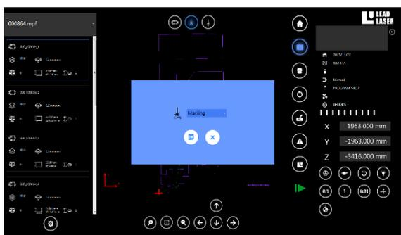
In the program information, the operator can graphically manipulate the cutting program without the need of the program software. Cutting or piercing technologies can be changed, and the cutting head movement between contours can be adjusted to the real situation on the machine if necessary for example to avoid any flipped parts. With one single button a program for a single part from
