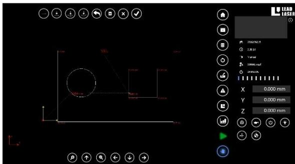
Simple programs can be made on the machine itself. An intuitive interface allows you to select graphical elements (lines and arcs) to draw simple parts. While programming the part in this graphical way, the part is drawn simultaneously indicating all relevant points and movements, so it is easy to detect mistakes and correct them immediately. Once the part is drawn, the relevant laser cutting and piercing technologies are selected and the machine code is generated, of course all automatically.
