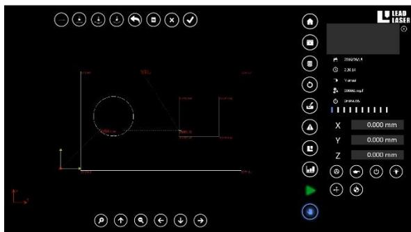
Simple programs can be made on the machine itself. An intuitive interface allows you to select graphical elements (lines and arcs) to draw simple parts. While programming the part in this graphical way, the part is drawn simultaneously indicating all relevant points and movements, so it is easy to detect mistakes and correct them immediately. Once the parts is drawn, the relevant laser cutting and piercing technologies are selected and the machine code is generated, of
