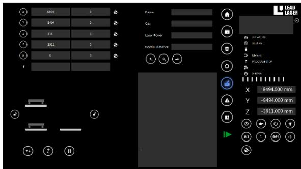
A more traditional machine interface screen shows all operation conditions of the machine together with the feed-back values from the integrated process sensors. An easy interface allows both manual and automatic operation of the shuttle table. At all times, the main features of the machine can be activated by the software control panel buttons on the right of the screen (and for left-handed operators: on the left of the screen).
