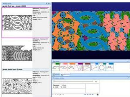
The PRC LEAD $\pi$ IIF-4020 can be delivered with Off-line software for nesting and programming. Libellula and PRC Lead Laser Suite<sup>©</sup> share a common database with all materials and thicknesses and their corresponding cutting and piercing technology parameters, allowing a simple one-button starting of each task on the machine. The configuration of all cutting and piercing technologies in Libellula is fully automatic and pre-defined for every Lead Laser machine.
