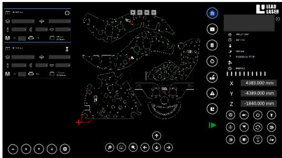
All tasks for the machine can be managed, organized and visualized in the task manager. PRC Lead Laser Suite<sup>®</sup> will provide the operator with all necessary information about the correct set-up of the machine. When used with automatic loading and unloading equipment, the task manager will make the work queues for full automatic operation of the laser cutting manufacturing cell.
