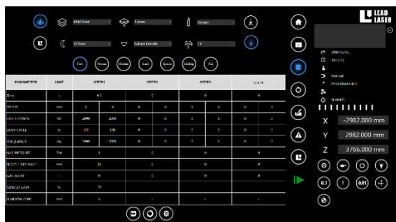
In PRC Lead Laser Suite<sup>®</sup> the parameters of all cutting and piercing technologies for every material and thickness are present on-board and can be managed in this dedicated page. Default values for all common applications are stored for reference in the Lead Laser database, the customer can create and add his own materials and parameters in the fully flexible and intelligent database manager.
