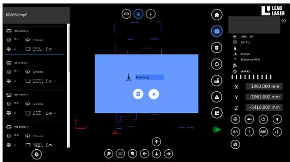
In the program information, the operator can graphically manipulate the cutting program without the need of the program software. Cutting or piercing technologies can be changed, and the cutting head movement between contours can be adjusted to the real situation on the machine if necessary for example to avoid any flipped parts. With one single button a program for a single part from
