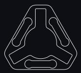
MATERIAL SHEET THICKNESS SIZE CUTTING LENGTH MILD STEEL 12MM 210MM X 287MM 1975MM
